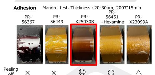
Thickness: 20-30um, 200°C15min Water resistance After dipping in hot water at 80°C for 12hr
