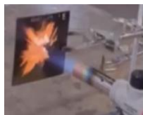
Torch burner test (800°C x 10min)
