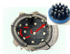
Resin-based flexible dry electrode
