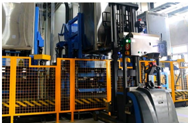
Self-activation of transport work using AGVs (Automatic Guided Vehicle)
