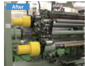
Measures to prevent entanglement in machinery (Amagasaki Plant)
