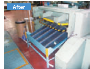
Measures to prevent entry into the cutting portion of shearing machinery (Kanuma Plant)
