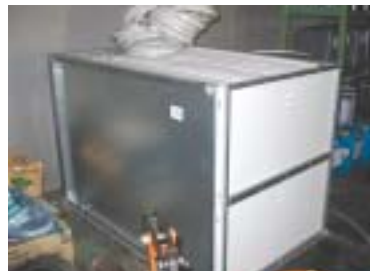
A recycling bin for fluorescent light bulbs
